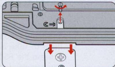
2. Loosen the silver screw on the inside of the camera back. Remove the battery chamber cover.
