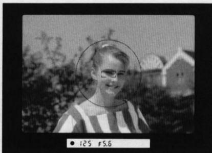
**2** Confirm that ● (in-focus indicator) appears in the viewfinder. Focus remains locked as long as you keep the shutter release button lightly pressed.
