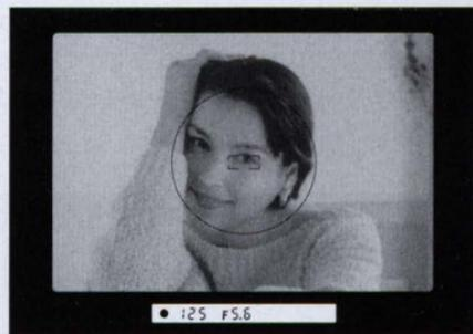
**2** Lightly press the shutter release button to activate autofocus operation and the exposure meter. Confirm ● (in-focus indicator) and exposure.
