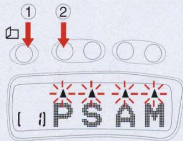
**2** Press the menu button ① to access the exposure mode menu, then press the button above P ②.
