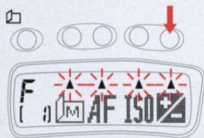
**1** With the Exposure Mode Menu, press the menu button to activate the Optional-Function Menu. Press the button above the
