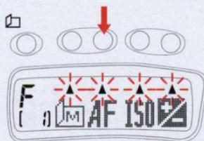
**1** With the Exposure Mode Menu, press the menu button to activate the Optional-Function Menu. Press the button above **AF**.
