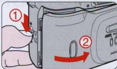
1. Make sure that film is not loaded, open the camera back.
