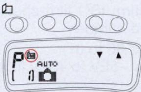
**4** Memory is set.
