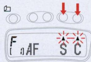
**2** For Continuous Servo AF, press the button above **C** for Single Servo AF, press the button above **S**. The LCD shows the last selected exposure mode/Program.
