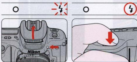
The flash can be used when the subject is within 0.6m to 3m when using a film with ISO 100 and the AF Zoom-Nikkor 35-80 mm f/4-f/5.6 D lens.
