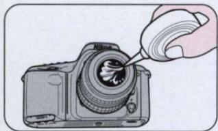
5. Clean glass surfaces, such as the lens or the eyepiece, with a blower brush; do not use lens tissue, silicon type eyeglass tissue, etc. To remove dirt and smudges, use soft cotton moistened with denatured alcohol and wipe surfaces in a spiral motion from centre to periphery. Do not leave traces.
