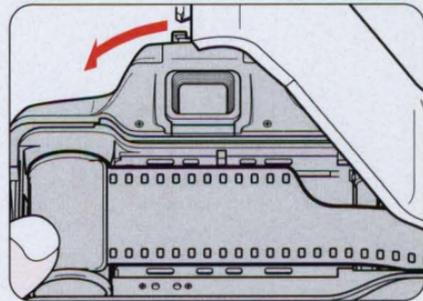
**4** Make sure the film is properly positioned with no slack and the film perforations engage the sprockets. (See illustration.)
