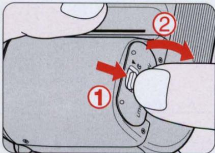
**1** Make sure the camera's power is off, then slide the lock release on the battery chamber cover to open the chamber.
