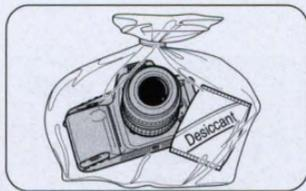
11. Store the camera in a cool, dry place away from naphthalene or camphor (moth repellent). In a humid environment, store the camera inside a vinyl bag with a desiccant to keep out dust, moisture and salt. Note, however, that storing leather cases in vinyl bags may cause the leather to deteriorate.
