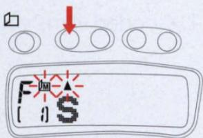
**3** The symbol for the selected exposure mode or Program is displayed. Press the button above the symbol to have it memorised.
