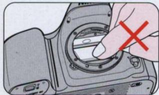
1. Do not touch the camera's reflex mirror or focusing screen. Remove dust with a blower brush.
