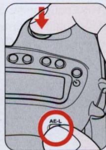
**4** While keeping the AE-L button pressed, recompose the picture, then fully depress the shutter release button.
