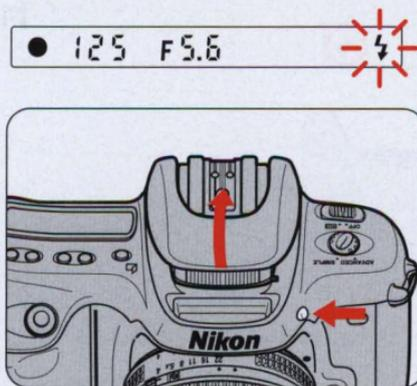
**1** When subject brightness is insufficient, the ready-light
