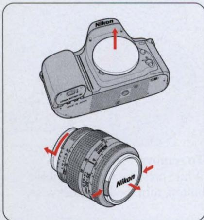
**1** Remove the camera body cap and the front and rear lens caps.
