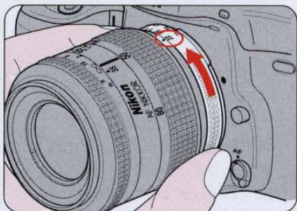
**3** Turn the lens aperture ring to its minimum aperture (the largest f-number, marked in orange, on AF Nikkor lenses). Then lock the lens aperture at its minimum setting (see lens instruction manual).
