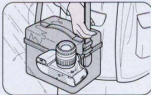
8. Keep the camera away from water or moisture. When using the camera near water, guard against splashes, especially salt water spray.
