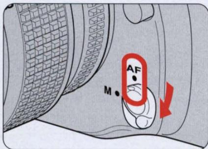
Autofocus should be used for most picture-taking situations, including moving subjects. In general, it is best to leave the focus switch set to AF.
