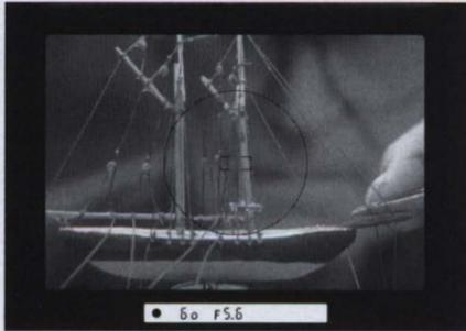
**6** Confirm that ● (in-focus indicator), the shutter speed (from 1/2000 to 30 sec.) and an aperture (number with **F**) appear below the viewfinder screen.
