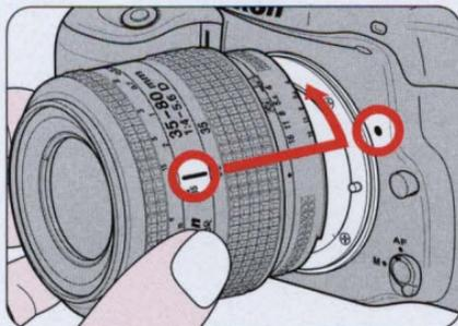
**2** Position the lens in the camera's bayonet mount so the mounting indices on the lens and the camera body are aligned. Twist the lens counterclockwise until it locks into place.
