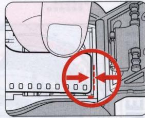
**3** Turn on the power switch and load film. Pull the film leader out to the red index
