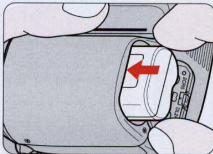
**2** Insert a 6V lithium pack with "+" and "-" ends positioned as shown on the inside of the cover. Close the cover by pushing until it clicks.
