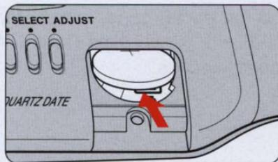
4. Insert new battery with "+" terminal facing upward.
