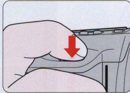
**7** Fully depress the shutter release button to take the picture. The film will automatically advance by one frame.
