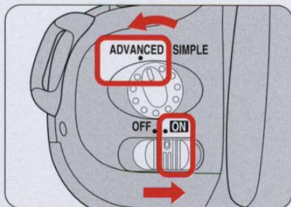
**1** Switch power ON and set the camera dial to ADVANCED. The LCD shows the last selected exposure mode/Program. (The original factory setting is for General-Purpose Program.)
