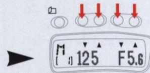
To change shutter speed/aperture rapidly, hold the button down.
