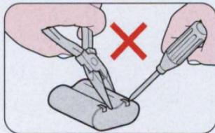
2. Do not disassemble, short circuit or heat batteries. Do not charge batteries.
