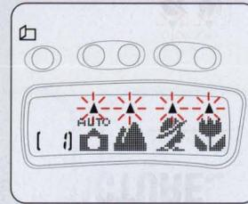
To select the General Purpose Program quickly Just press the menu button for at least two seconds.
