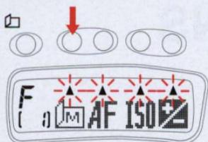
**1** With the Exposure Mode menu, press the menu button to activate the Optional-Function Menu. Press the button above
