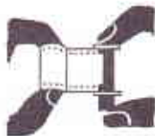
Right: Inserting the loaded spool into the cassette.
