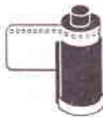
Below: Cassette inserted in the Exakta for cassette-to-spool use. (Exa is similar, but with feed cassette on the left.)
