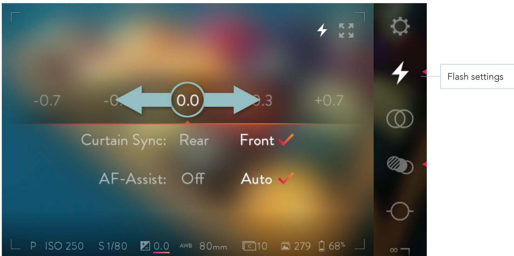
*With the Viltrox JY680L TTL flash mounted to the ILLUM hot shoe and powered on, touch the Flash icon to open the flash control interface. Swipe left or right to adjust TTL compensation values. Tap again to close the control interface.*
