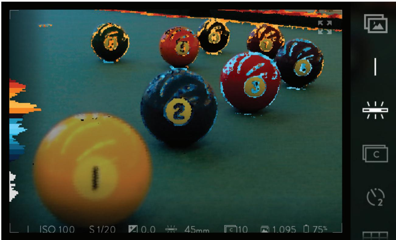
Objects in the near refocusable range are edged in blue; those in the far refocusable range are edged in orange. White in the histogram represents the elements in the scene which will be outside the refocusable range in your Living Picture, and can not be focused on when interacting with the image.
