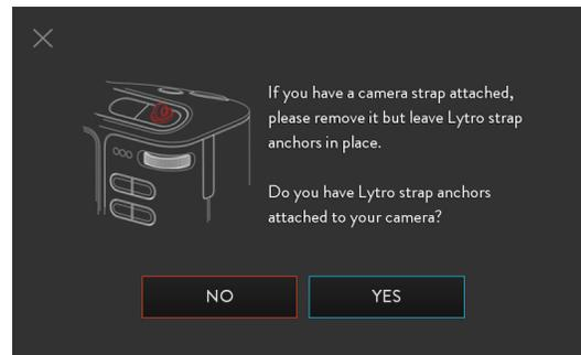
Follow the on-screen guide to calibrate the ILLUM level. You must remove the ILLUM lens hood and camera strap before calibrating. If you have attached the Lytro strap anchors to the ILLUM, click YES when prompted. If you have not attached the Lytro strap anchors, click NO. The 6 step calibration process is ready to start.
