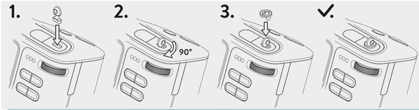
Once strap anchors are installed, attach the strap using the split-rings.
