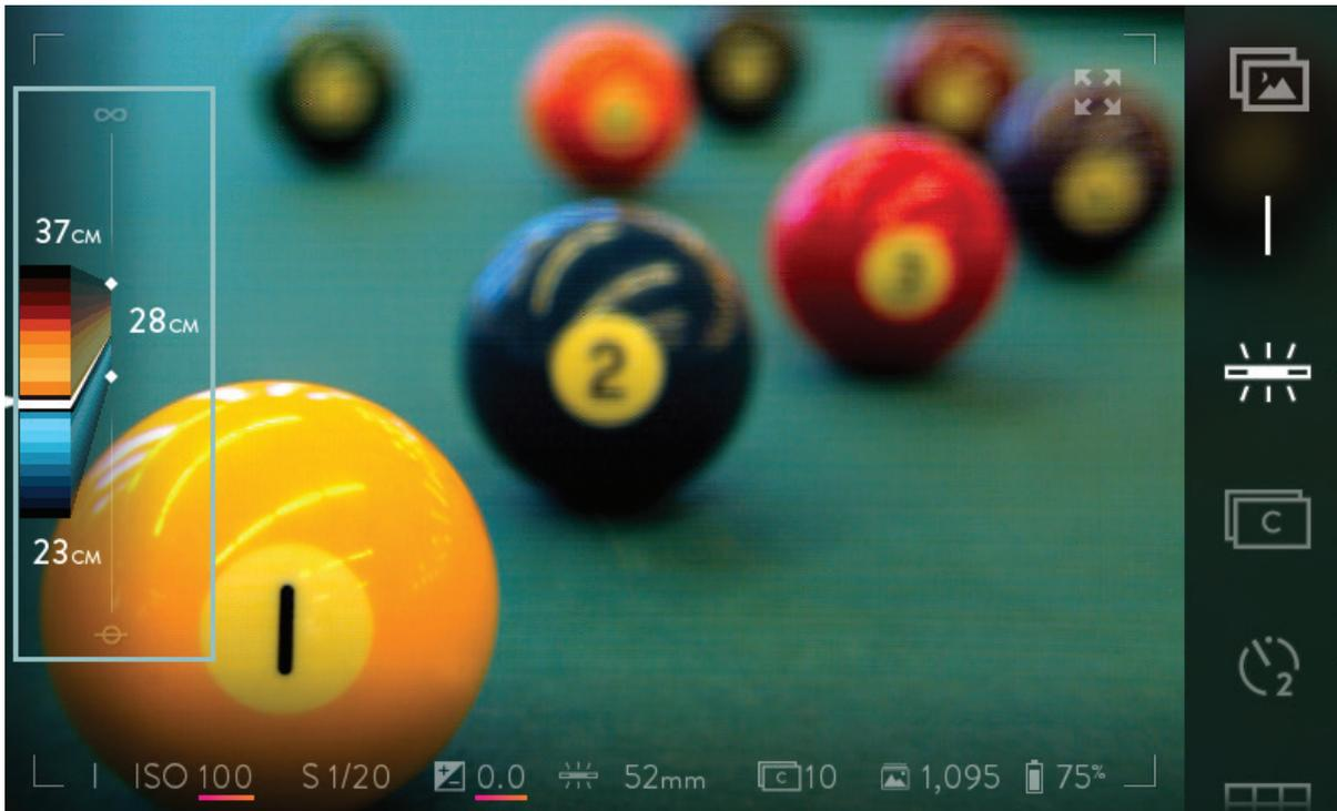
*In the Depth Assist Bar, the orange and blue bands, or Depth Steps, represent the refocusable range. The numbers indicate the physical distances from the camera.*
