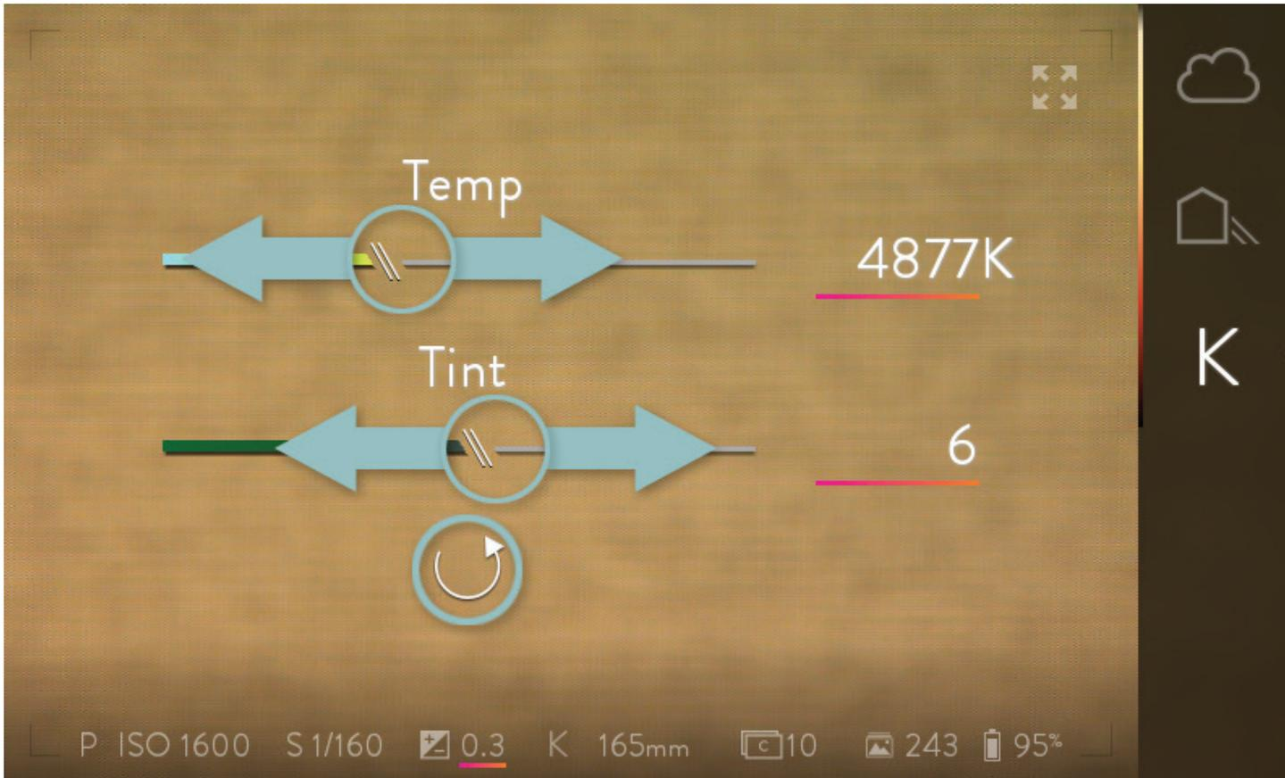
*Tap the sliders and sweep side to side to adjust their values. Tap the counter clockwise arrow to revert to the original Manual White Balance.*
