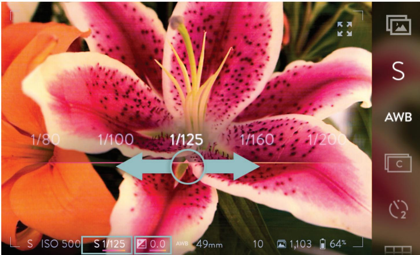
*Swipe the shutter speed selection band to increase or lower the speed.*
