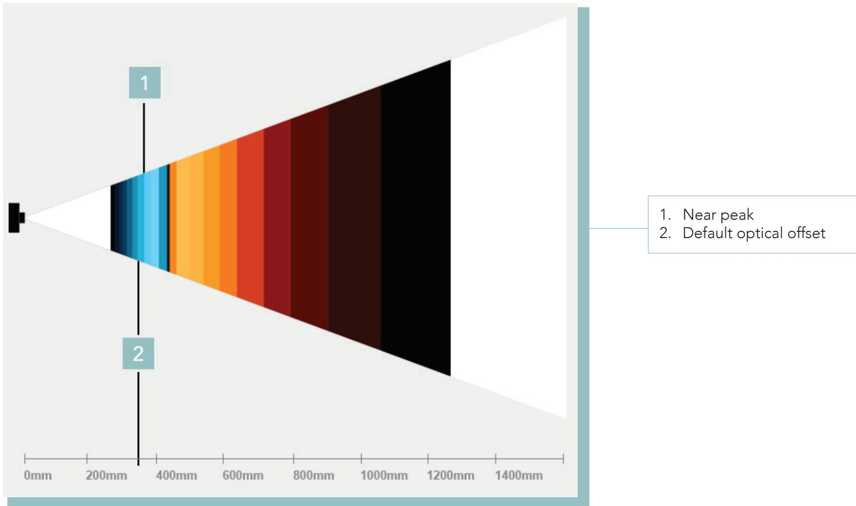
*The default optical offset, with the focus position used for the live view and for autofocus set at the peak of the near refocusable range*
