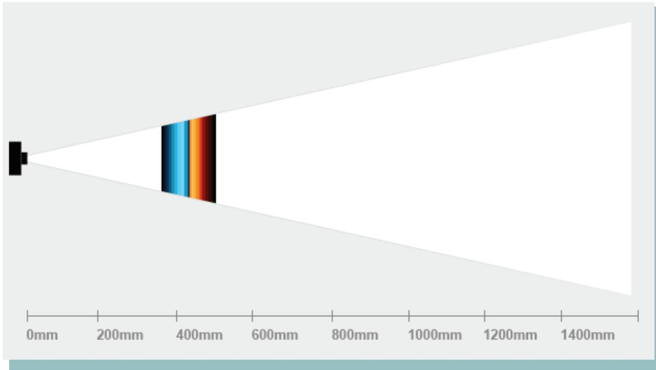
*The refocusable range with the lens zoomed to a 100mm focal length (35mm equivalent) and the optical focus at approximately 42cm. Note the relative size of the refocusable range.*
